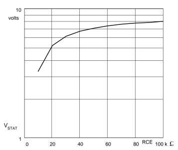
Fig.7b V<sub>CEstat</sub> as function of R<sub>CE</sub>
