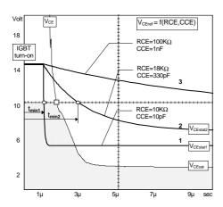
Fig.6 V<sub>CEref</sub> waveform with parameters R<sub>CE</sub>, C<sub>CE</sub>
