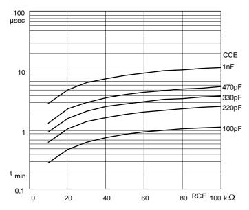
Fig.7a  $t_{min}$  as function of  $R_{CE}$  and  $C_{CE}$
