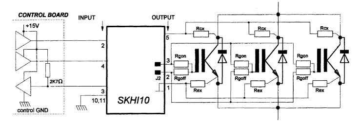
Fig. 9 Preferred circuit for paralleled IGBT's
