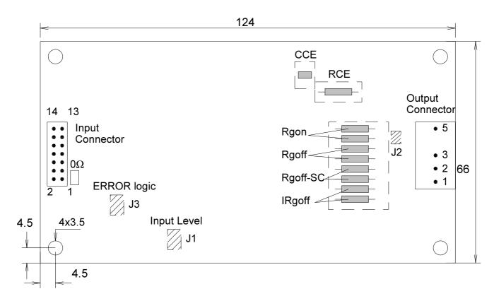
Input connector = 14 pin flat cable according to DIN 41651
