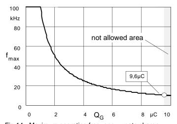
Fig.14 Maximum operating frequency x gate charge
