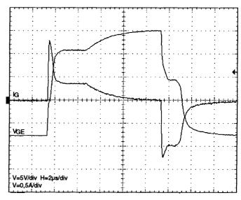
Fig. 11 Output voltage (V<sub>GE</sub>) and output current (I<sub>G</sub>)
