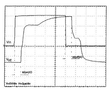
Fig. 10 Input and output voltage propagation time
