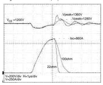
Fig.13 Effect of R<sub>goff</sub>-SC in short - circuit
